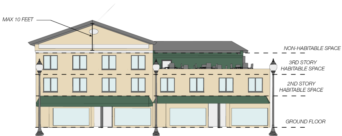
Figure B.12.2 Building Height Illustrations
