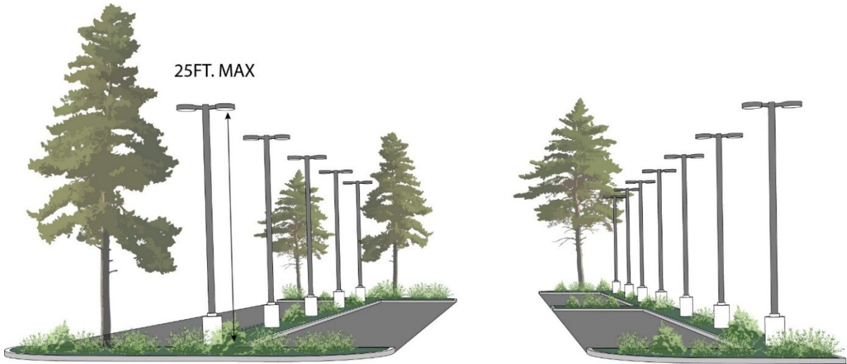
Figure C.4.3 Parking Area Lighting
