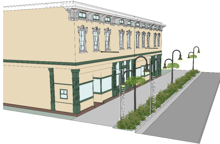
Figure C.4.2 Light Fixture Height
