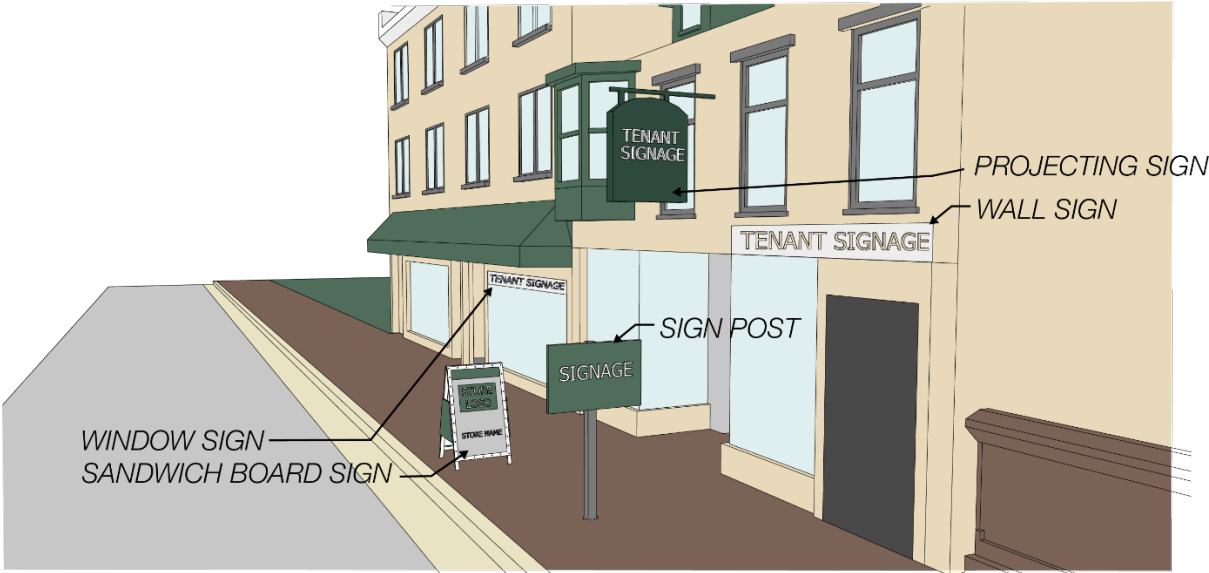
Figure C.3.13 Illustrative Example of Building Signs
