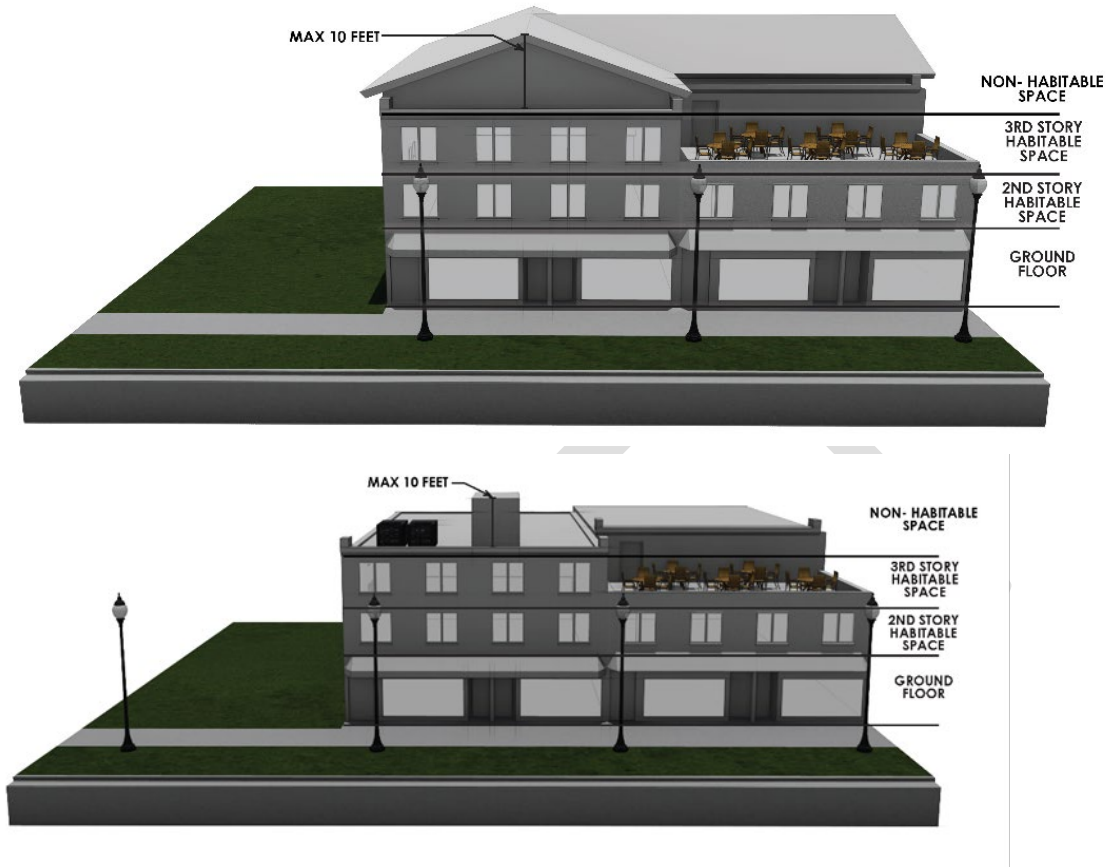
Figure B.10.2 Building Height Illustrations
