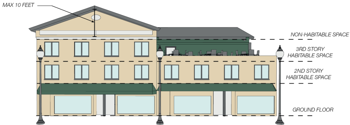
Figure B.12.2. Building Height Illustrations
