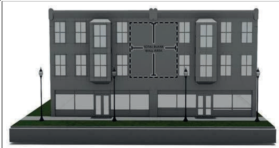
Figure B.11.2 Blank Wall Area
