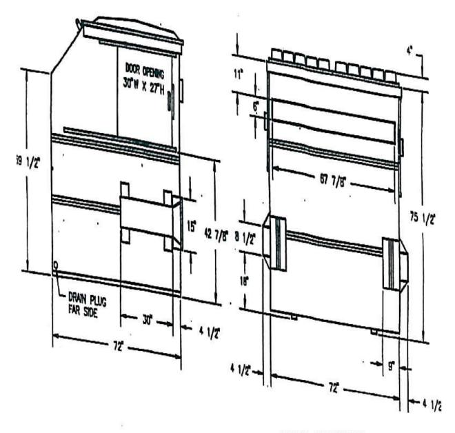
MATERIAL SPECIFICATIONS: -SIDES 12 GA. -BOTTOM 10 GA. -SLEEVES 7 GA. -TOP CHANNEL & RUNNERS C3 X
