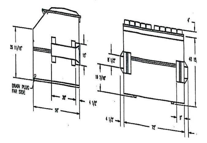
MATERIAL SPECIFICATIONS: -SIDES 12 GA. -BOTTOM 10 GA. -SLEEVES 7 GA. -TOP CHANNEL & RUNNERS C3 X
