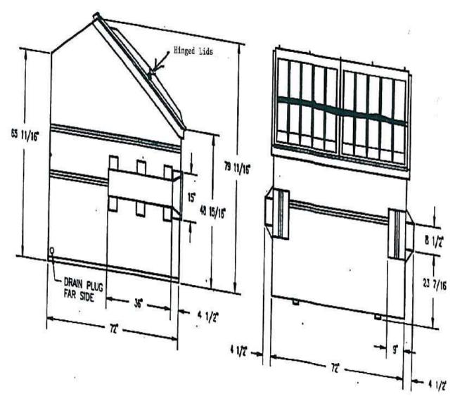
MATERIAL SPECIFICATIONS: -SIDES 12 CA. -BOTTOM 10 GA. -SLEEVES 7 GA. -TOP CHANNEL & RUNNERS C3 X
